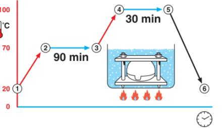
**GB** ① Start curing process in cold water + Increase water temperature ② Start curing + Maintain water temperature ③ Increase water temperature ④ Start curing + Maintain water temperature ⑤ Stop curing + Air cooling to ambient temperature ⑥ End of total curing process
